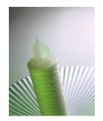
POLIXSTER ADM FREE is obtained by pleating together up to 4 polyester layers of decreasing porosity to achieve high effective filtration area, high dirt holding capacity and controlled filter ratings.
